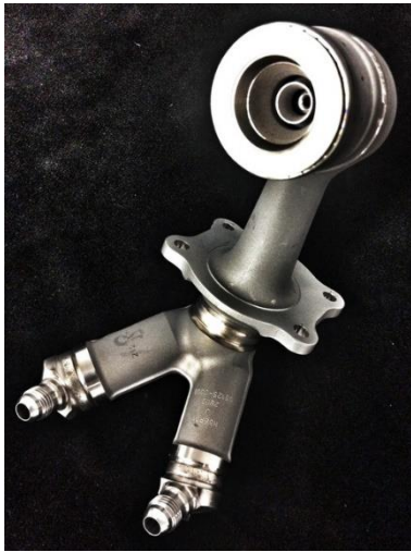
3D printed fuel nozzle for LEAP engine (GE)
